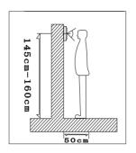
Indoor unit Standard installation height is 145cm~160cm (distance between screen centre and the floor)
