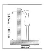
Indoor unit Standard installation height is 145cm~160cm (distance between screen centre and the floor)
